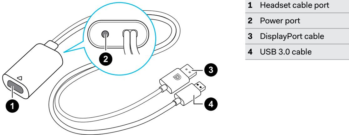
1. Connect the power adapter cable to its corresponding port on the converter for VIVE Cosmos Elite.
