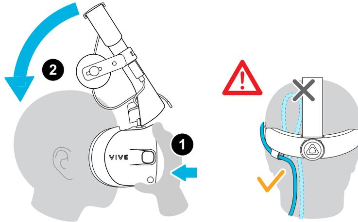
4. Pull down the headset band around the back of your head until you hear a click. The click indicates that the headset band has locked into place.
