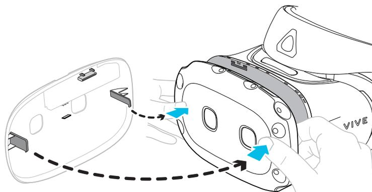
6. Press the right side of the front cover first, and then press the left side of the front cover.
