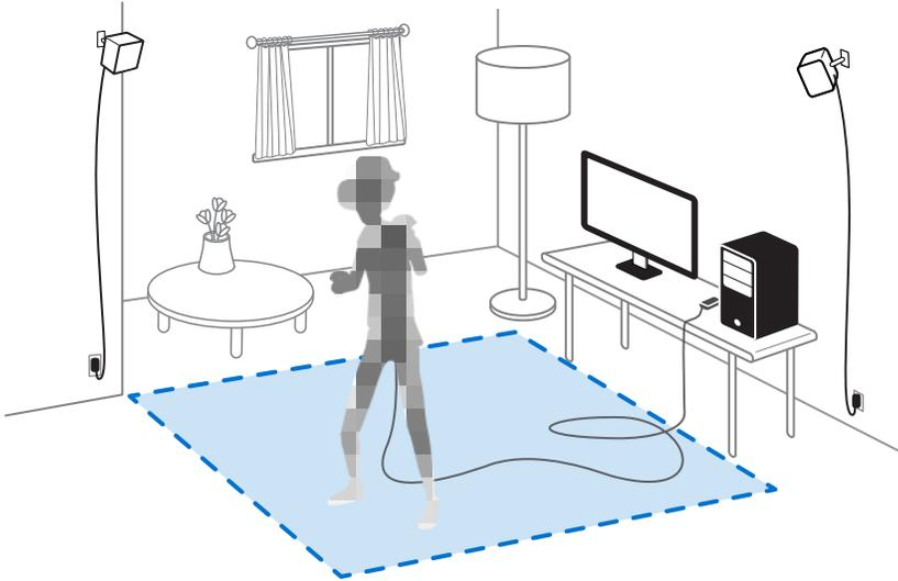
While you're in the play area, the headset and the controllers should remain at least 0.5 m (1 ft 7 in) and no further than 5 m (16 ft 4 in) away from a base station. This will ensure that the devices are properly tracked within the base station's 120-degree field of view.
