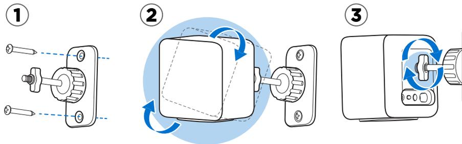
4. To adjust the angle of the base station, loosen the clamping ring while carefully holding the base station to prevent it from falling.
