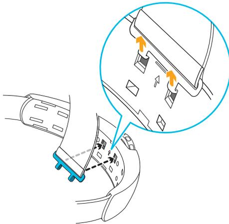
3. Align the back pad tabs with their corresponding slots on the band, and then press along the back pad to reattach. You'll hear a click when the tabs are inserted.
