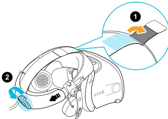
2. While holding the visor with one hand, pull up the band.
