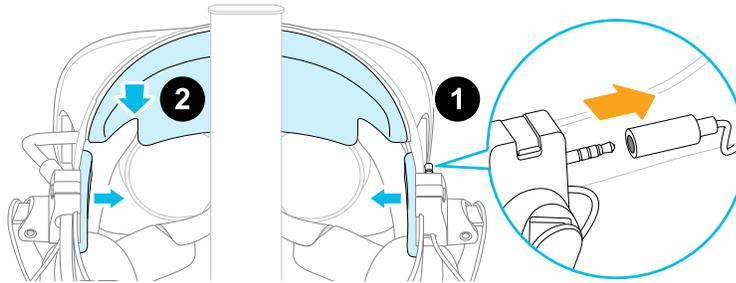
3. On the front section of the band, carefully pull out the cable of the on-ear headphones from the groove.
